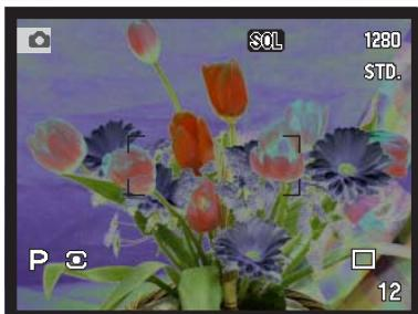
**Solarization** – produces a partial reversal of tones in the image. The Digital Effects Control's exposure compensation function can be used to accentuate the solarization effect (p. 67). Contrast, saturation, and filter adjustments cannot be made. This color mode does not affect RAW images.
