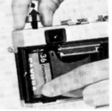
3. When there is a sudden drop in the pressure felt in your hand and the film rewind button stops turning, open the back cover and take out the cartridge.
