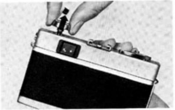
1. Flip up the Film Rewind Crank (6) and forcibly pull it up, and the Back Cover (18) will open and the film counter will indicate the mark "S" (start).
