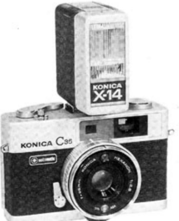
When you use an X-14, clip it into the accessory clip of your camera, and your camera will shift from EE to flash photography as long as the guide number is set to 45 (when film with ASA ratings from 80 to 125 is used). The aperture will be automatically adjusted in conjunction with focusing.
