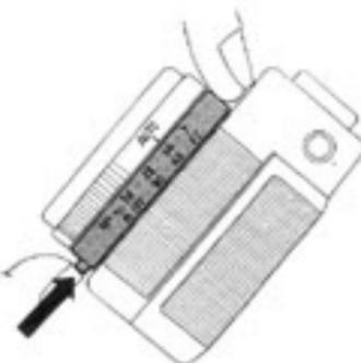
2. If some object other than an accessory is inserted into the accessory clip the camera will be automatically set to flash exposure. So do not try to put into the clip anything other than a flash or electronic flash unit.
