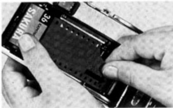
3. Insert the film tip into the slit of the Film Take-up Spool (17). The film tip can be inserted into any slit.
