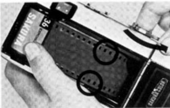
4. Turn the Film Wind Lever (3) and ascertain that perforations on both sides of film are in gear with the film Sprocket (16), before the back cover is closed.
