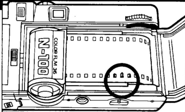
**5** Close the back cover while pressing the film cassette up against the top of the film chamber.
