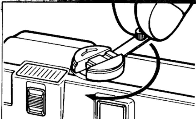
**7** Alternately wind on film and shoot blank shots until the exposure counter reads "1". While winding on the film, check that it is advancing properly by observing whether or not the film rewind knob turns.
