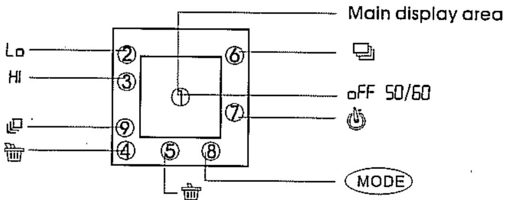
Press the select button to select the functions on the digital camera. The function diagram will show on the LCD display:
