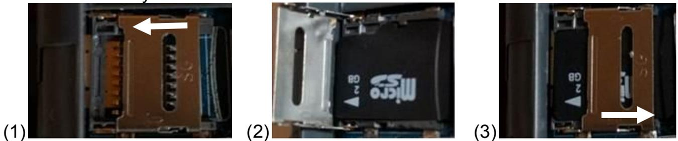
**Tip: If the memory card does not work, check that it is inserted correctly and also check the metal contact points. You can also try to format the memory card. You shouldn't have to close the metal clip with a lot of strength.**
