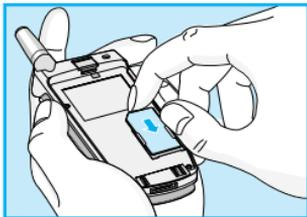
1. Remove the battery if attached.
