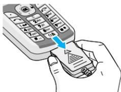
Disconnect the travel adapter from the phone by pressing its side buttons as shown in the diagram.
