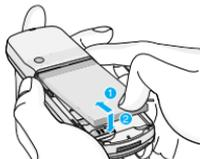
1. Position the lugs on the top of the battery into the retaining holder.
