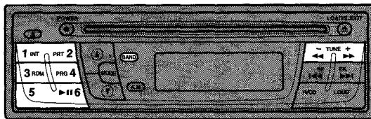
Up to 6 stations for each band [FM1, FM2, FM3, and AM] can be stored on the preset station buttons.
