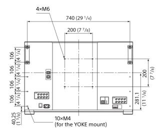
To install on a vehicle, fix the unit using screw holes for the YOKE mount.
