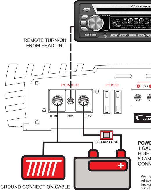
SHOULD USE SAME GAUGE WIRE AS POWER CABLE. KEEP GROUND CABLE AS SHORT AS POSSIBLE. ALL AMPLIFIERS IN A MULTI-AMP INSTALLATION SHOULD GROUND TO THE SAME LOCATION TO AVOID GROUND LOOPS.
