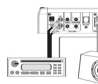
Configuration and C GTA-500m Amplifier Powering a Subwoofer
