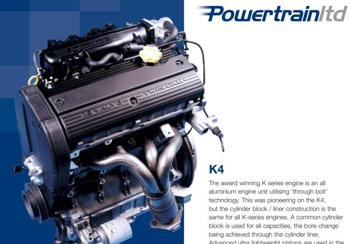
The award winning K series engine is an all aluminium engine unit utilising 'through bolt' technology. This was pioneering on the K4, but the cylinder block / liner construction is the same for all K-series engines. A common cylinder block is used for all capacities, the bore change being achieved through the cylinder liner. Advanced ultra lightweight pistons are used in the 1.8 unit, resulting in reduced second order inertia forces for improved engine refinement.
