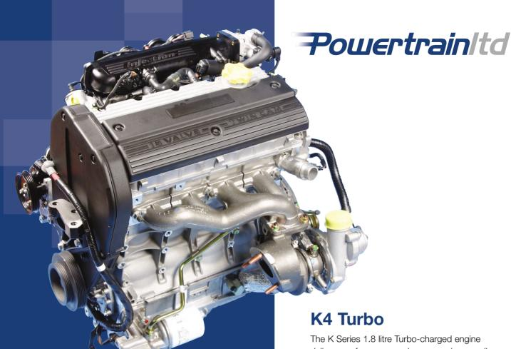
The K Series 1.8 litre Turbo-charged engine delivers performance and economy in a small package. The engine incorporates the latest developments in broad range turbocharger technology where aerodynamic improvements give a much a wider range of operation. These changes give both reduced back pressures at high speeds and loads as well as improved rotor acceleration at low speeds. The result is a responsive turbo charged engine with very good low speed torque, fuel economy and CO2 emissions.
