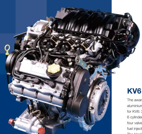
The award winning K Series engine is an all aluminium unit available in two capacity variants for KV6: 2.0 litre and 2.5 litres. The engines are 6 cylinder water cooled, naturally aspirated with four valves per cylinder and utilising multi-point fuel injection with sequential operating capability. The block and liner construction is common across the range. all have direct acting overhead camshafts and hydraulic tappets, with toothed belt drive via an auto tensioning system.
