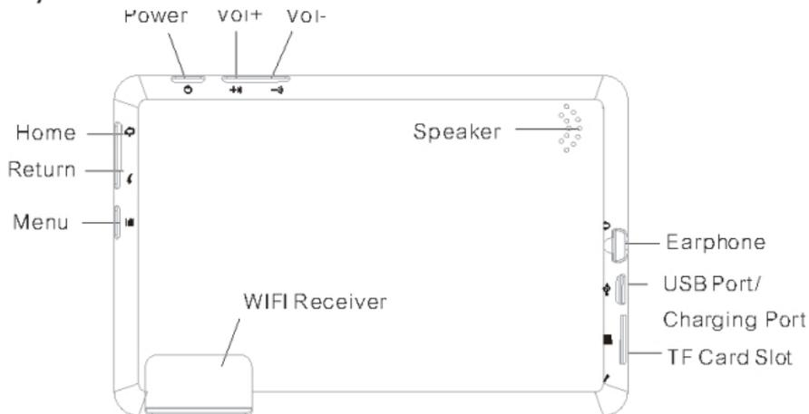
**There are five function keys located on the machine surface.**
