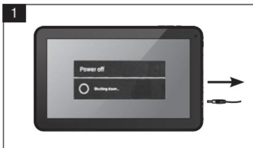
**1b** Be sure to disconnect the power adapter plug out of the tablet, but leave or place the adapter itself in the wall socket.
