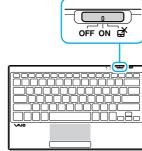
Set the power and touch pad on/off switch for Keyboard to ON.
