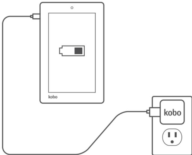
Charge by connecting to a power source.
