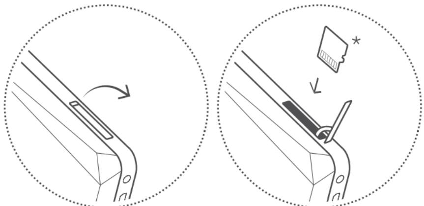
Lift tab to insert a Micro SD card.
