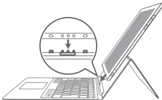
Make sure that the keyboard is aligned with the slots, and attach your MateBook E to the keyboard properly.
