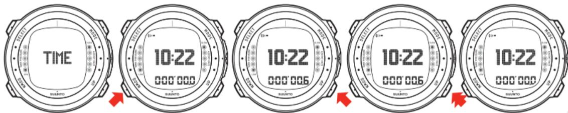
UTILISEZ LE BOUTON DOWN POUR LANCER LE CHRONOMÈTRE ET PRENDRE UN TEMPS INTERMÉDIAIRE. LE BOUTON UP ARRÊTE LE CHRONOMÈTRE. SI VOUS AVEZ PRIS DES TEMPS INTERMÉDIAIRES, VOUS POUVEZ LES FAIRE DÉFILER PAR UN APPUI BREF SUR LE BOUTON UP. UN APPUI LONG SUR LE BOUTON UP REMET LE CHRONOMÈTRE À ZÉRO.
