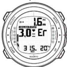
PLONGEE AVEC PALIER DE DECOMPRESSION, AU-DESSUS DU PLAFOND. UNE FLECHE POINTEE VERS LE BAS, UN SIGNAL ER ET UNE ALARM. VOUS DEVEZ IMMEDIATEMENT (DANS LES 3 MINUTES) DESCENDRE AU PLAFOND OU PLUS BAS.
