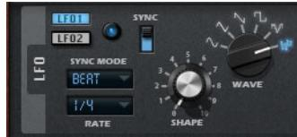
Retrologue features two monophonic LFOs. In this context, monophonic means that the LFOs are calculated once and feed multiple voices at the same time. You switch between the settings for LFO 1 and LFO 2 by clicking the corresponding button.
