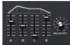
The Velocity control determines how much the envelope intensity depends on velocity. When the control is set to 0, the envelope is fully applied. Higher values reduce the intensity for lower velocities.
