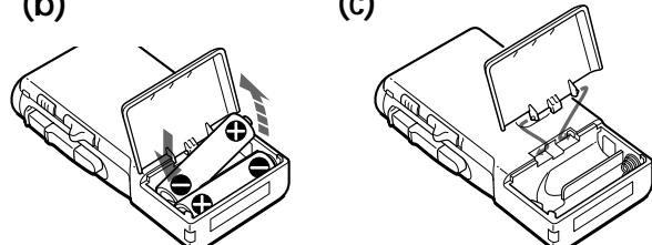
**To take out the batteries (see Fig. A-(b))****If the battery compartment lid is accidentally detached (see Fig. A-(c))**
