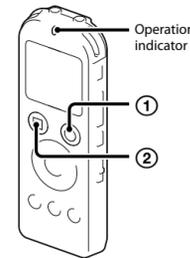
Before you start using the IC recorder, make sure that you slide the HOLD-POWER switch towards the center to release the HOLD status.
