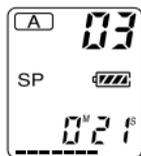
2 While playing back the message, press FILE to flash the indication of the file to which you want to move the message (B in this case). The first and last 5 seconds of the message will be played back 10 times, while the file indication and "MOVE" flash.
