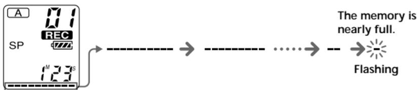
When the remaining time of recording reaches 5 minutes, the last one of the indication flashes. When the remaining time of recording reaches 1 minute, the selected display mode (page 34) and "REMAIN" will flash one after the other in the display window. When the memory is full, recording automatically stops and "END" will flash in the display window with an alarm sound. To continue recording, first erase some of the messages (page 18).
