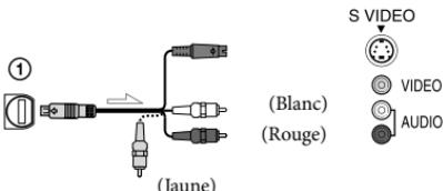
Câble de raccordement A/V (fourni)
