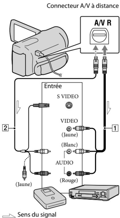
[1] Câble de raccordement A/V (fourni)
