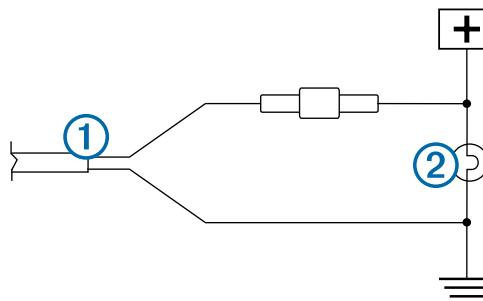
**NOTE:** Connecting the transmitter to an always-on 12–24 VDC source (such as a running lamp) instead of a reverse lamp requires you to manually switch power to the transmitter. The transmitter may drain your vehicle battery if it is left on.
