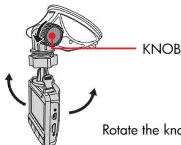
Rotate the knob to swivel the device vertically.
