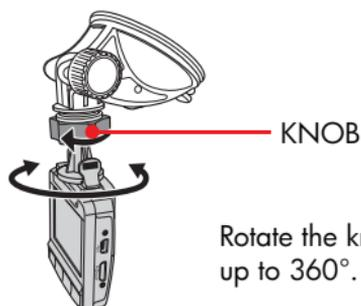
Rotate the knob to swivel the device horizontally up to 360°.
