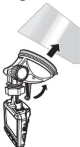
With the suction-cup laying flat, position the suction-cup on the windshield.
