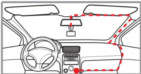
Connect the car adapter to the power connector of the Mobile Camera and then plug the other end to the vehicle's lighter socket.
