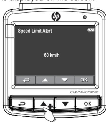
Press ▲/▼ button to set the speed limit. You can set the speed limit from 50km/h to 200 km/h.
