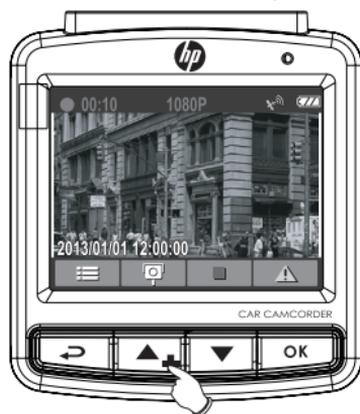
Press the ▲/⊕ button to add a speed cam point.
