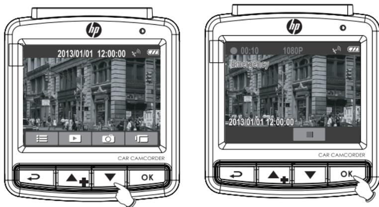
During Video Recording, press the OK button to enter emergency recording mode, the “Emergency” message will be shown immediately on the upper left corner of the screen, and the recorded file will be protected. If the Collision Detection function is enabled and a collision is detected, the device will automatically trigger the emergency recording feature.
