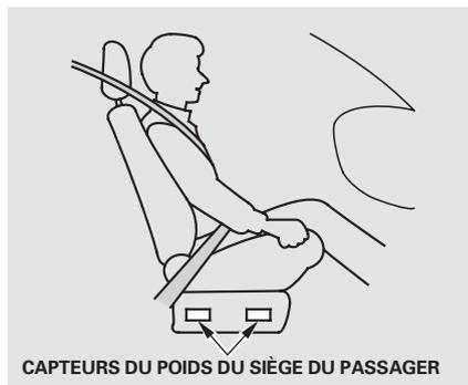
**CAPTEURS DU POIDS DU SIÈGE DU PASSAGER**
