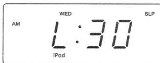
3.) To change the amount of **Sleep** time depress and hold the Sleep button and press the **Tuning/Skip**  $\blacktriangle$  or  $\blacktriangledown$  buttons on the top panel or the  $\blacktriangleleft/\blacktriangleright$  buttons on the remote control to decrease or increase the amount of sleep time from "**01**" minutes to "**99**" minutes.
