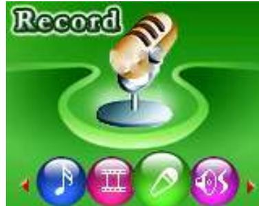
Press the [MENU] button again to start voice recording in WAV format (as shown in below image). Press the [▶||] button to pause the recording. Press and hold the [Menu] button to save the recorded file and return to the recording interface.
