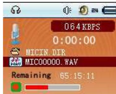
During the process of recording, short press [▶||] button will pause/ start recording, long press [Menu] button to save the recorded file and return to the playing interface.
