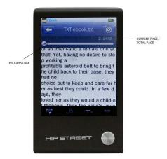
Manual/Auto Page Turning. The text will stop in manual mode; slide left/right to turn to the previous or next page. Auto mode means timed Auto Page Down, and the timing range is 3s, 6s, 9s, 12s, and 15s.
