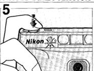
Lightly press the shutter release button and confirm that the viewfinder indicator LED lights up for a second, indicating battery power is sufficient.
