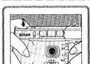
The built-in flash fires automatically when light is insufficient.
