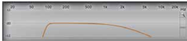
Crossover frequency 80 - 2000 Hz @ 48 dB/Oct. Hi-pass 2000 Hz @ 6dB Oct. Low-pass
