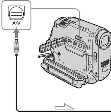
Câble de raccordement A/V (fourni)\*1
